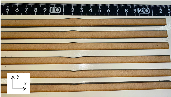
Fig. 6. Actual wooden bumps and dents used in Experiment 2. Three bumps and dents with different height/depth and width; their maximum gradients were equal.
