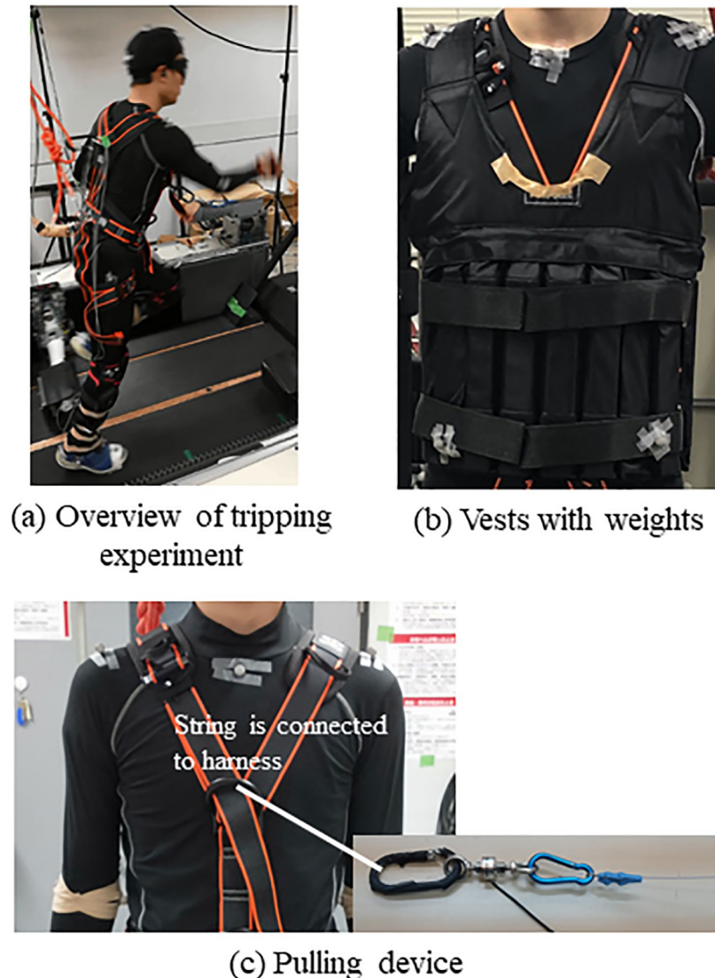
Fig 1. Experimental setups. (a) Overview of tripping experiment (b) Vests with weights (c) Pulling device.
